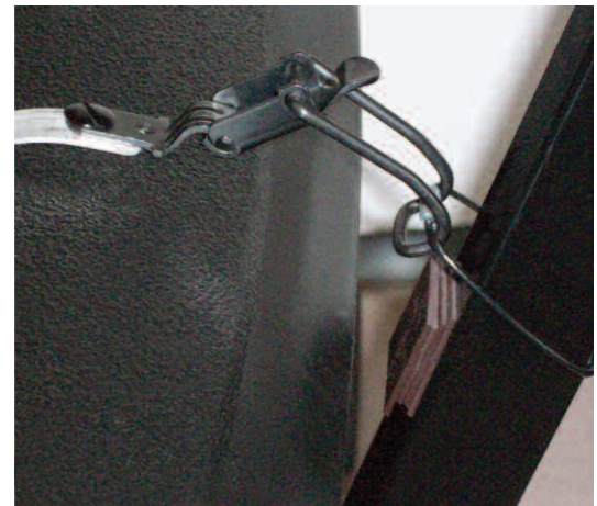
4 SHIMS IN PLACE, READY TO CLOSE LATCH
