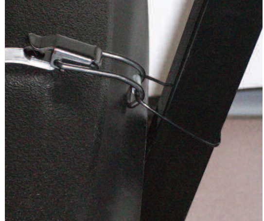
LATCHED WITH SMALL GAP BETWEEN T-BAR & SEAT
