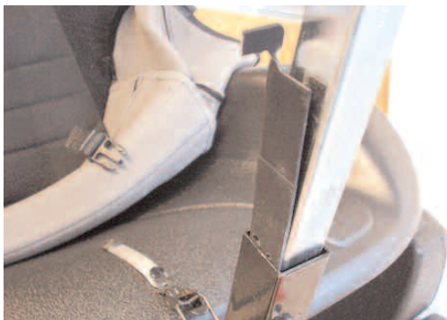
SIDE SHIM IN POSITION
