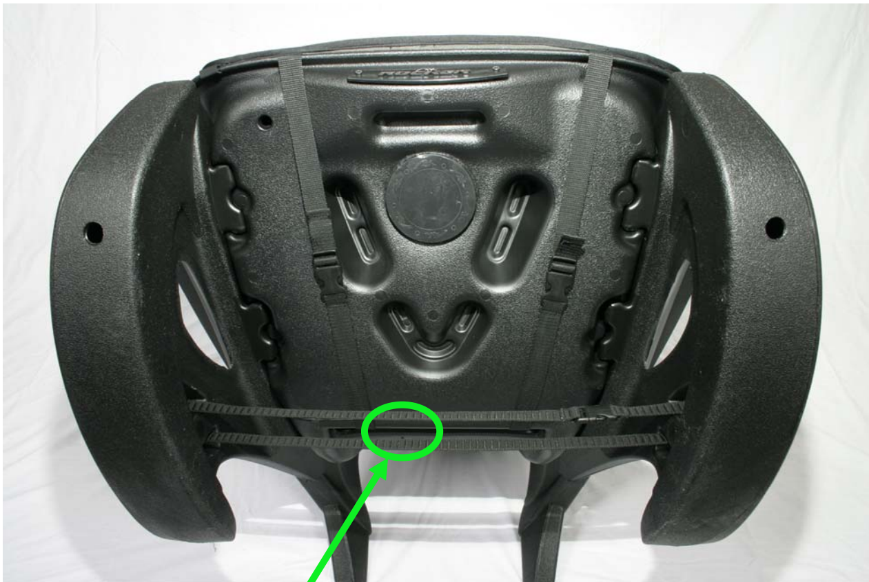
PowerStrap installed and hanging loosely
